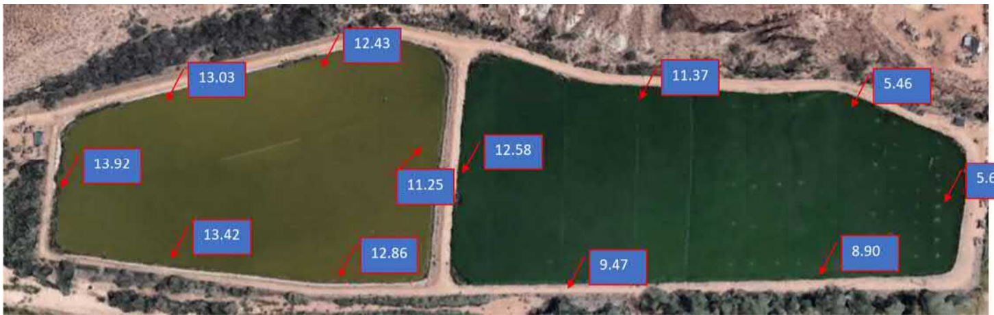
Figure 9. Dissolved Oxygen Locations Before Sunrise at the Springdale Wastewater Lagoon System. Sampled from 7:00 to 7:45 AM on January 22, 2020. Water Temperature Averaged 4.8 degrees C
