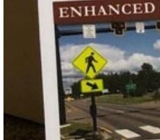
HIGH VISIBILITY CROSSWALK WITH FLASHING BEACON AND OPTIONAL AUDIO SIGNALS
